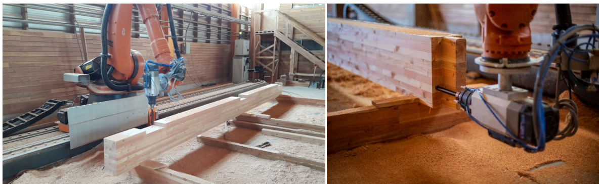
Figure 4: Box and dowel mechanization, Voipir, Villarrica, 2020
